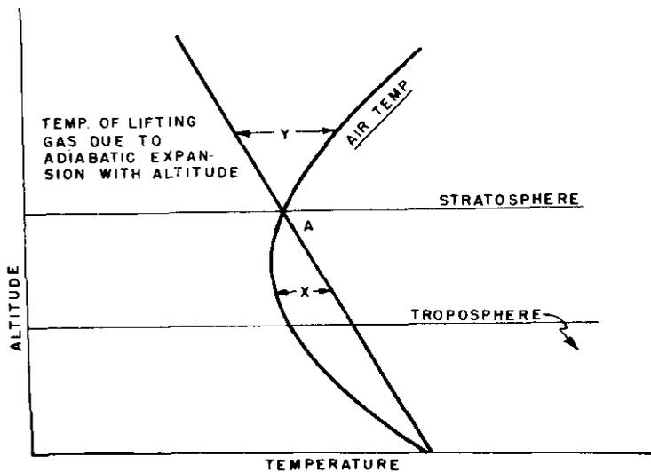
Figure 22. Lapse rate of air and helium.
