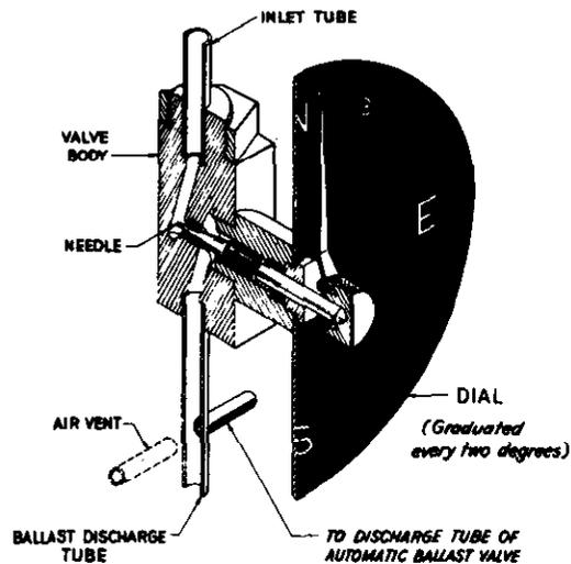
Figure 9. Manual ballast valve.
