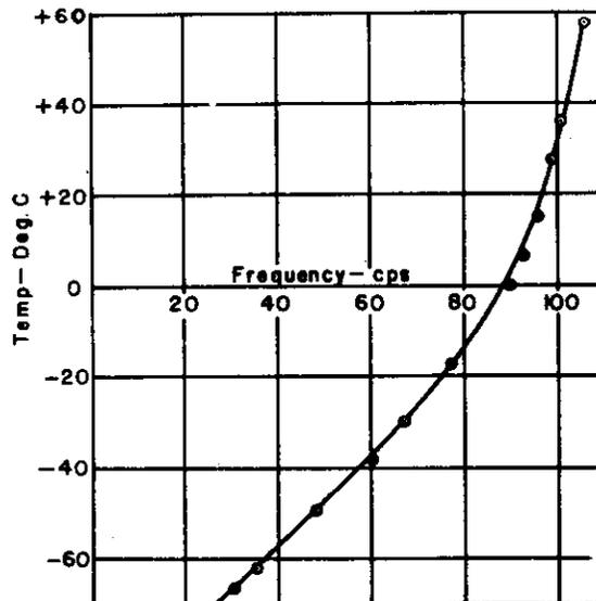
Figure 34. Sample calibration chart for temperature measurements.
