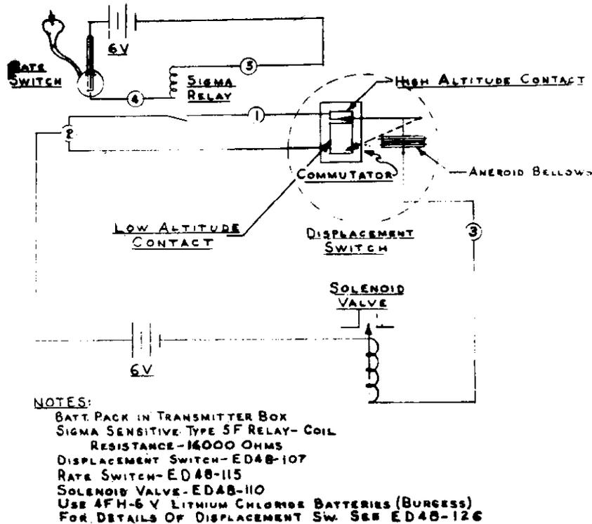
Figure 14. Circuit for ballast control with combined displacement and rate-of-ascent switches.
