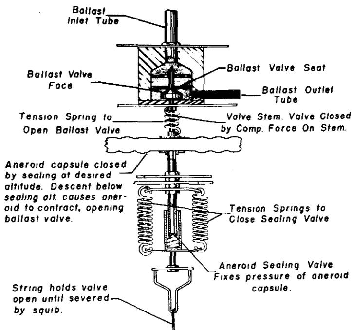
Figure 10. Automatic ballast valve.
