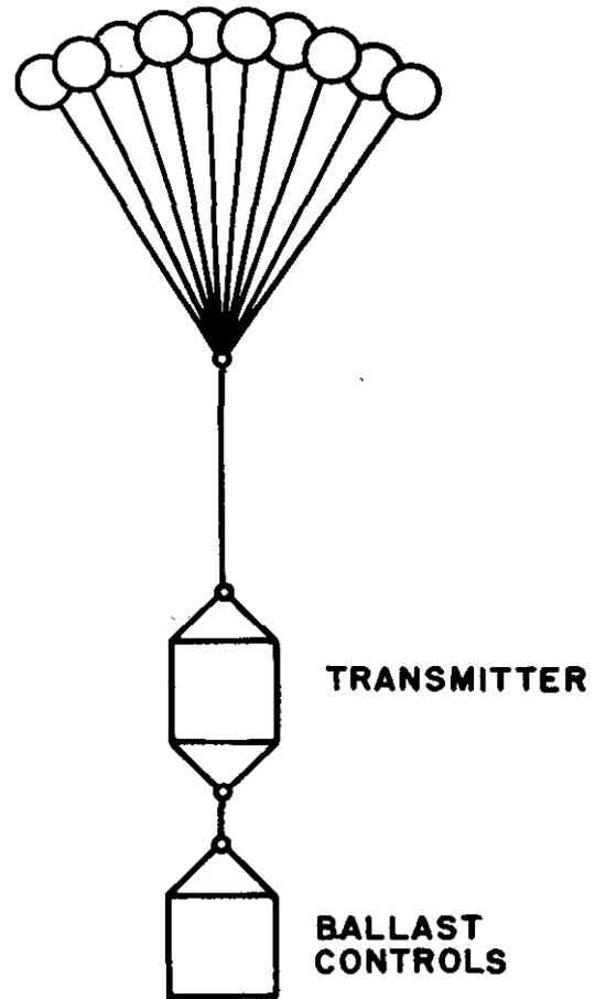
Figures 3 and 4. Typical rubber balloon arrays.
