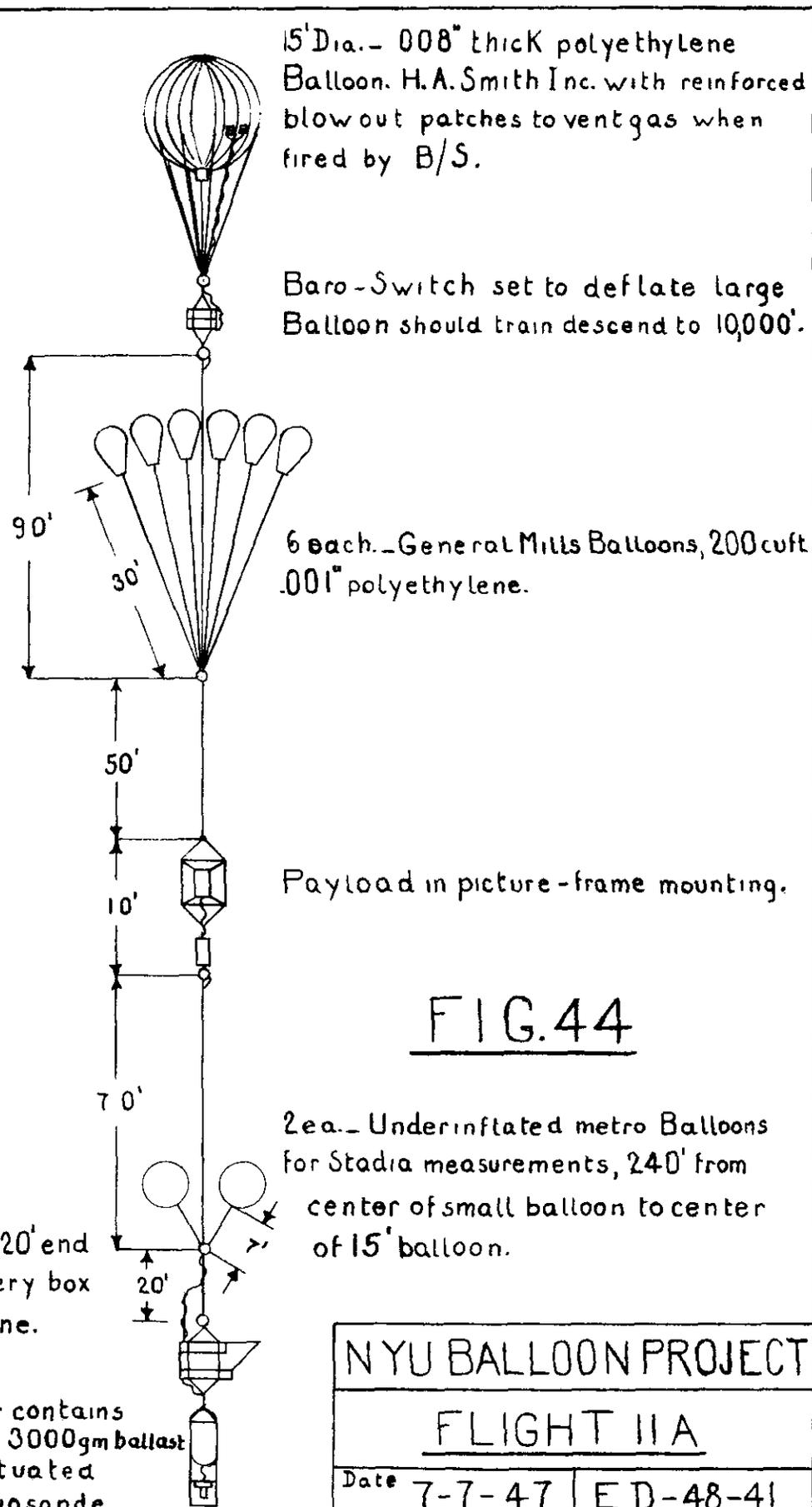
15' Dia. - .008" thick polyethylene Balloon. H.A. Smith Inc. with reinforced blow out patches to vent gas when fired by B/S.
