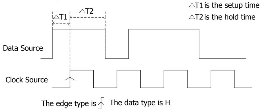
Figure 5-11 Setup/Hold Trigger
