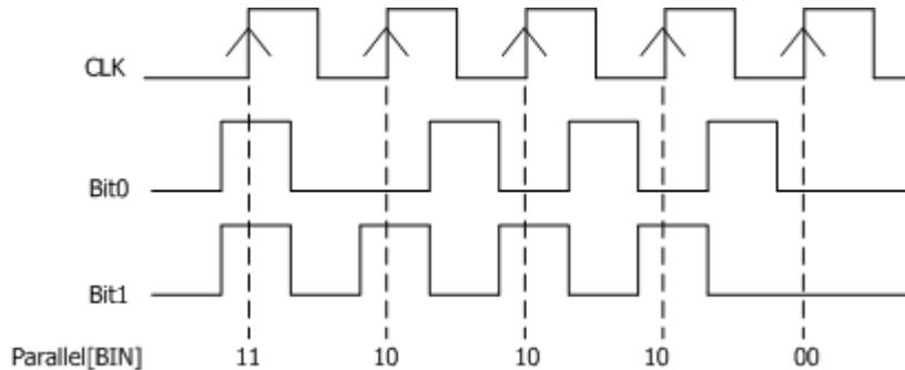
Figure 7-1 Parallel Decoding
