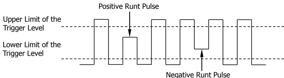
Figure 5-9 Runt Trigger
