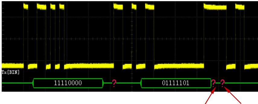
Frame Check Error      Frame End Error
