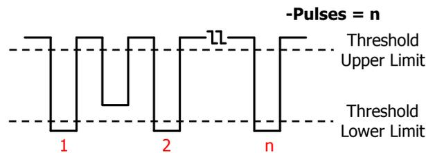
3. **+Edges:** the number of rising edges that rise from below the threshold lower limit to above the threshold upper limit.
