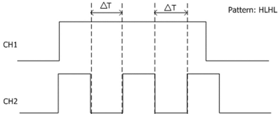
Figure 5-7 Duration Trigger
