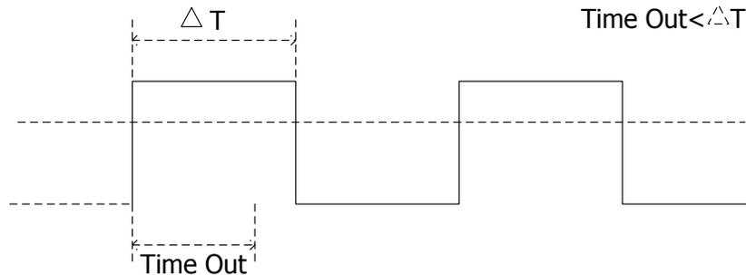
Figure 5-8 TimeOut Trigger
