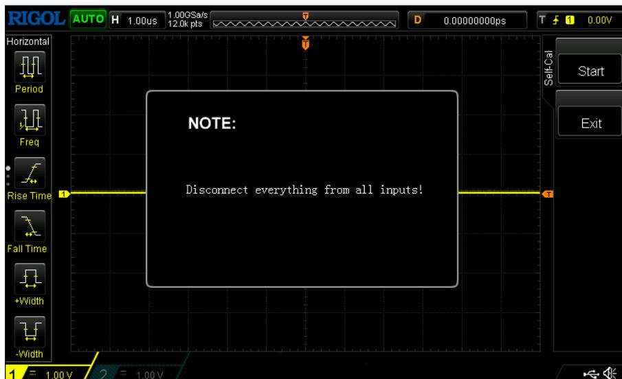
Figure 13-2 Self-calibration Interface
