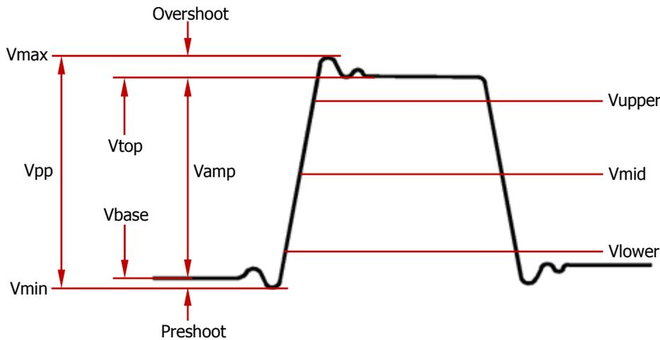
Figure 6-5 Voltage Parameters
