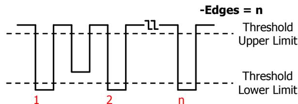
**Note:** The default values of the threshold upper limit and threshold lower limit are 90% and 10% respectively. You can set them via **Measure** → **Setting** → **Type** → "Threshold" and for the setting method, please refer to the introduction in "**Threshold Measurement Setting**".
