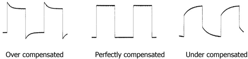
Figure 1-8 Probe Compensation
