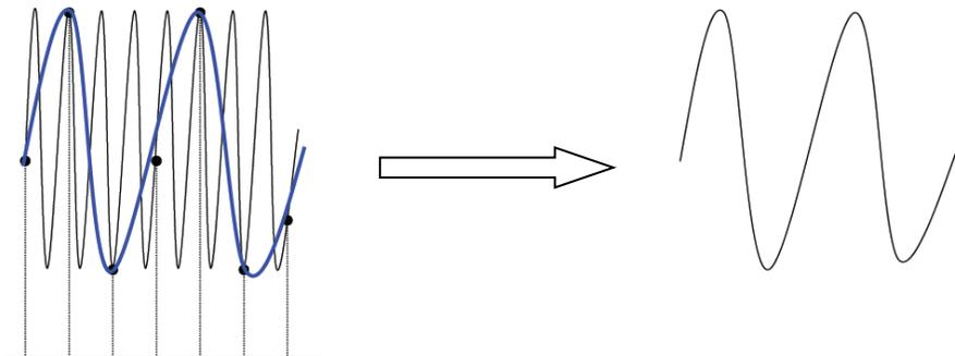
3. **Waveform Leakage:** when the sample rate is too low, the waveform rebuilt from the sample data does not reflect all the actual signal information.
