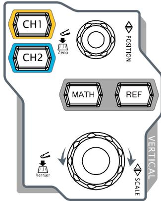
**CH1**, **CH2**: analog channel setting keys. The 2 channels are marked by different colors which are also used to mark both the corresponding waveforms on the screen and the channel input connectors. Press any key to open the corresponding channel menu and press again to turn off the channel.
