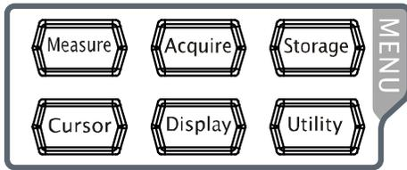
**Measure**: press this key to open the measurement setting menu. You can set the measurement source, turn on or off the frequency counter, all measure, statistic function and etc. Press **MENU** at the left of the screen to open the measurement menus of 37 waveform parameters. Then, press down the corresponding menu softkey to quickly realize one-key measurement and the measurement result will be displayed at the bottom of the screen.
