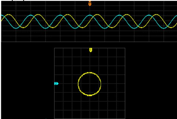
5. Observe the measurement result shown in the figure above. According to the measurement schematic diagram of the phase deviation (as shown in Figure 3-2),  $A/B$  ( $C/D$ ) = 1. Thus, the phase deviation angle  $\theta=\pm\arcsin 1=90^\circ$ .
