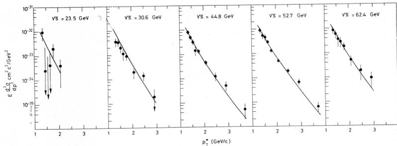
Fig. 7. The charge-averaged invariant cross section for electron production, plotted as a function of the c.m. momentum  $p_T^*$  for five values of  $\sqrt{s}$ . The curve represents a fit of the charge-averaged pion data of the BS Collaboration [22], and has been multiplied by  $10^{-4}$ .
