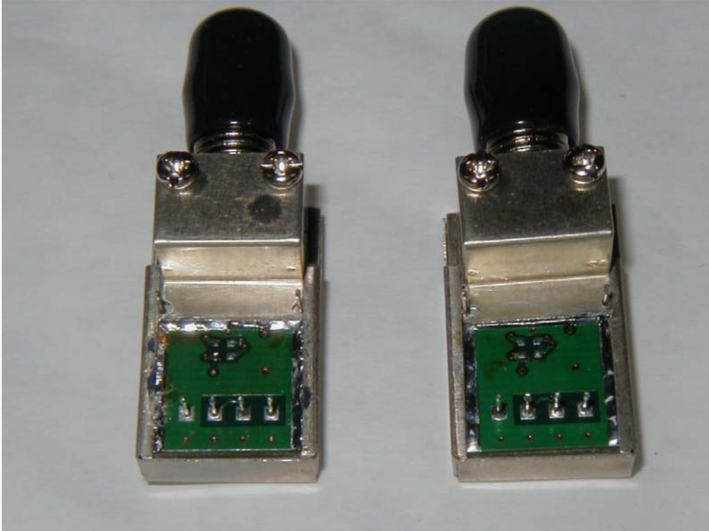
**Figure 2** The photo of two custom-made optical transmitters
