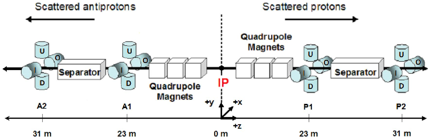
⇒ There are eight quadrupole spectrometers (Up, Down, In, Out) on the outgoing proton (P) and anti-proton (A) sides each comprised of two detectors (1, 2)
