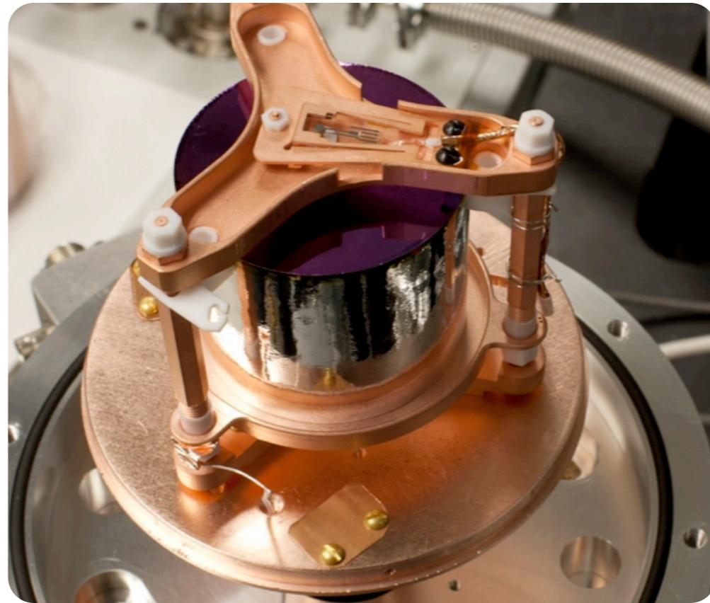
Diodes in vacuum cryostats
