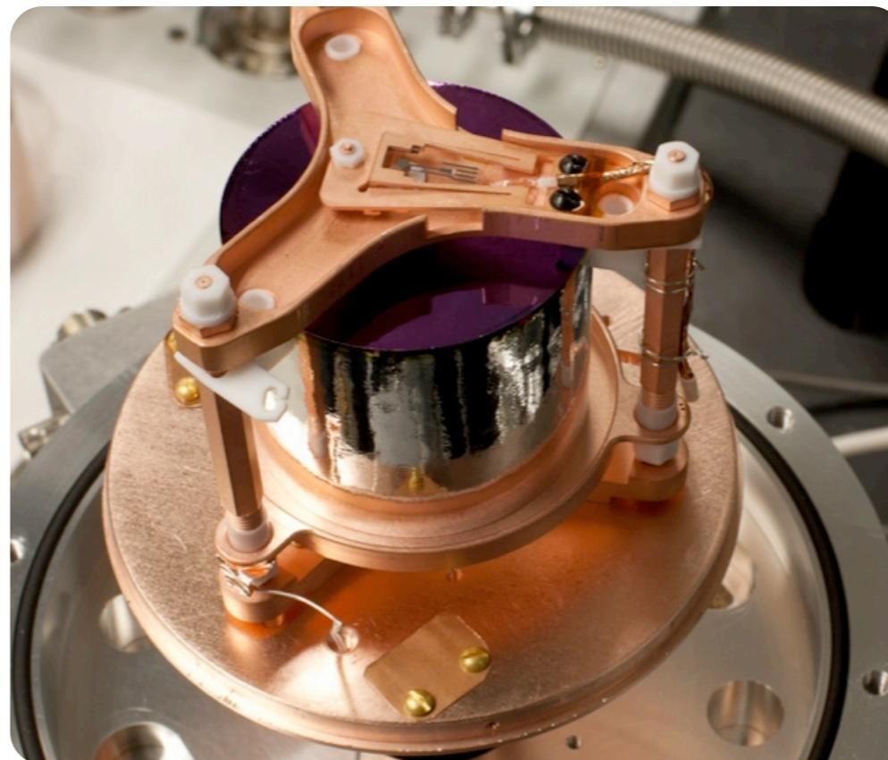
Diodes in vacuum cryostats
