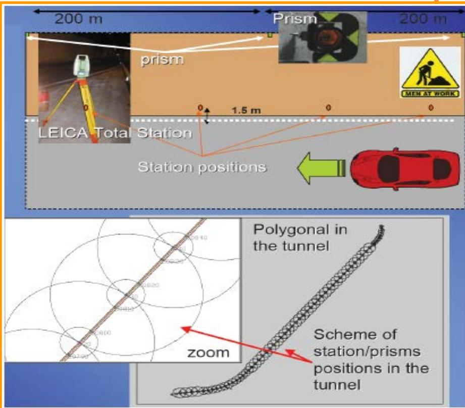
→ Geodesy measurements to link the OPERA detector position underground to GPS benchmarks
