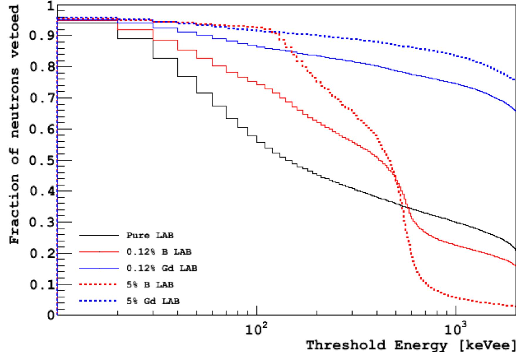
Veto efficiency vs threshold for 100 $\mu$ s veto times for recoil events.
