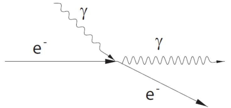
Collision of low energy photons with relativistic electrons
