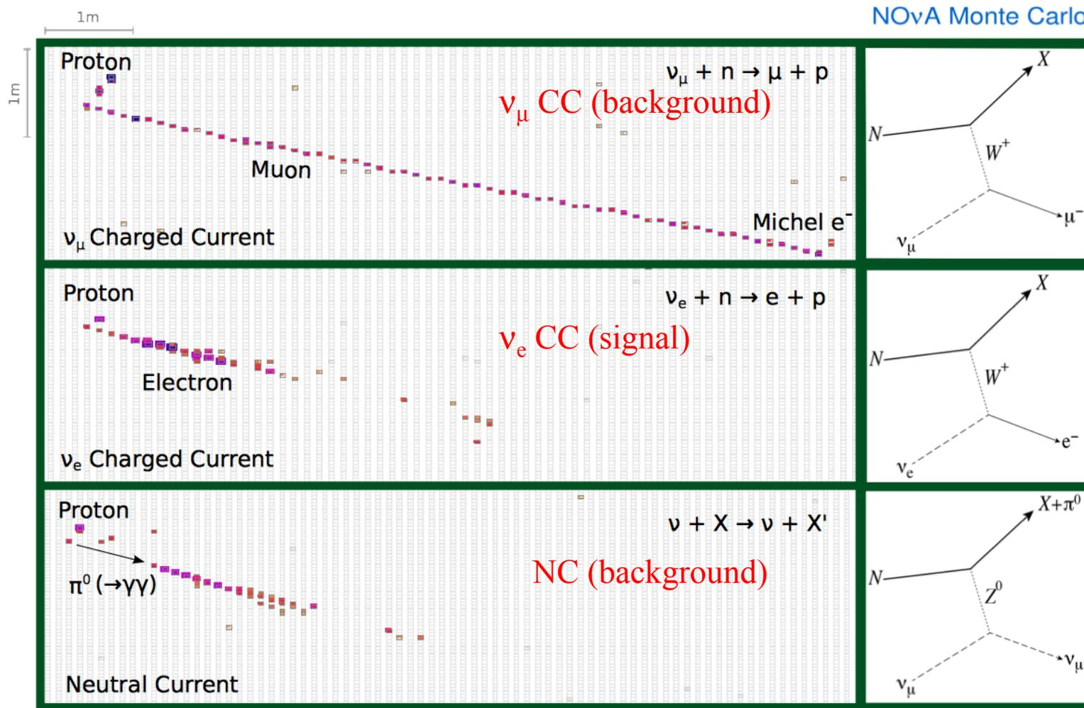
The **muon** is a long minimum ionizing particle (MIP) track, the **electron** ionizes in the first few planes then starts a shower and the **photon** is a shower with a gap in the first few planes.
