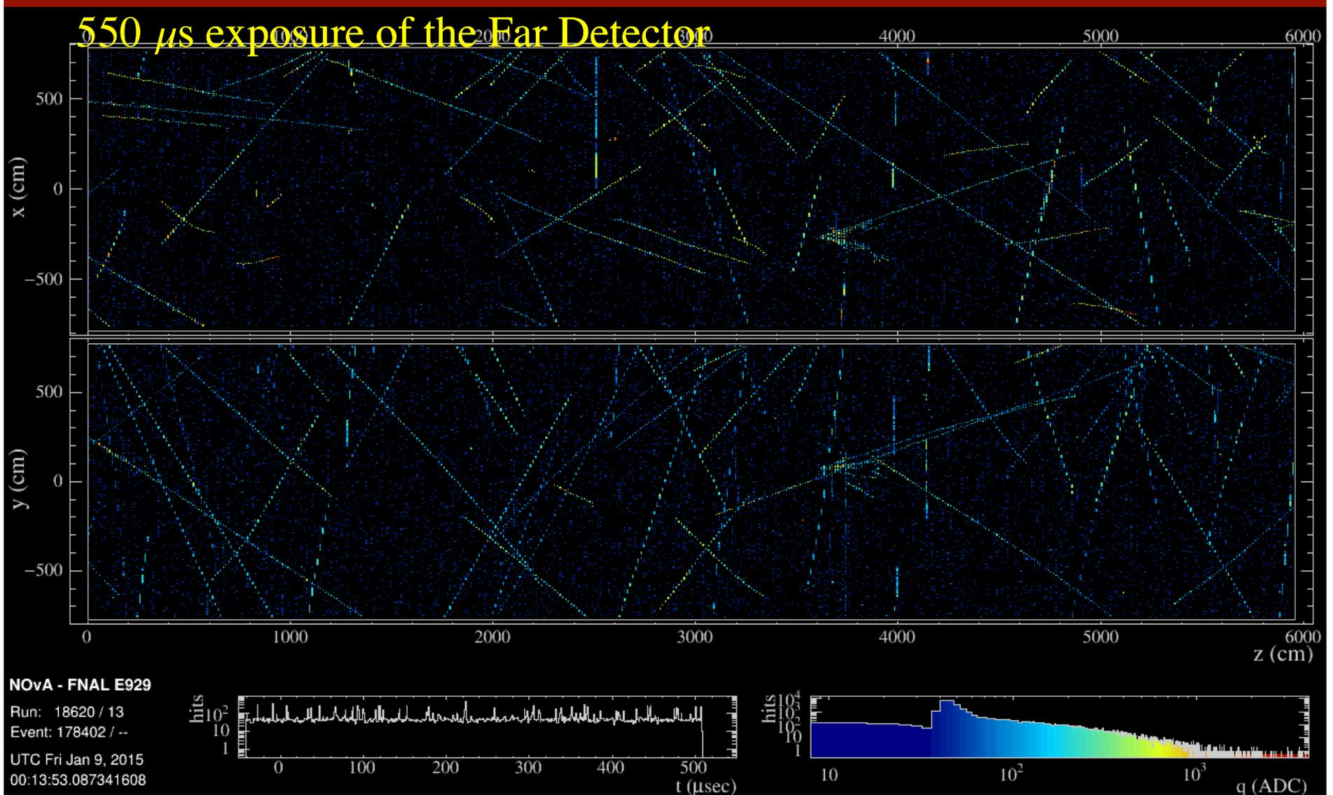
Because hits in a 550 $\mu$ s trigger window are a combination of cosmic and beam events, first step in reconstruction is to cluster hits by space-time coincidence
