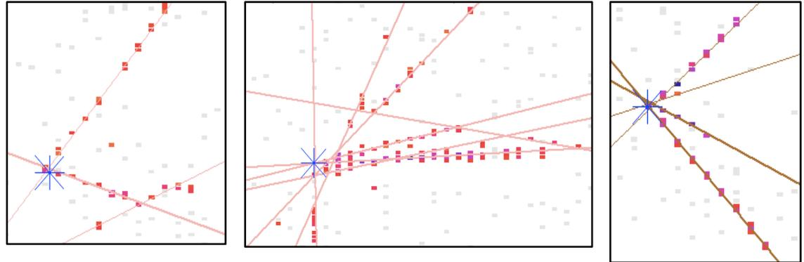
**Shower Clustering:** Based on the vertex, prongs are determined by angular clustering.
