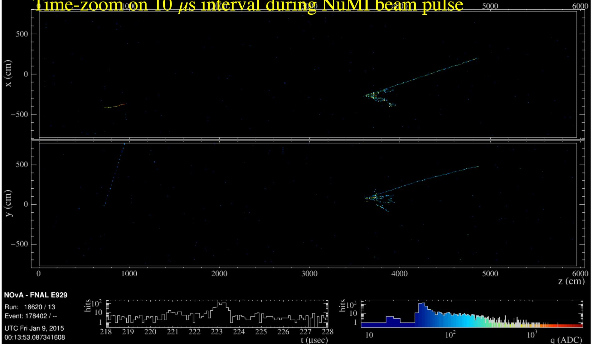
Event clusters that contain neutrino interactions can be correctly selected in the in the 10 $\mu$ s neutrino spill timing window
