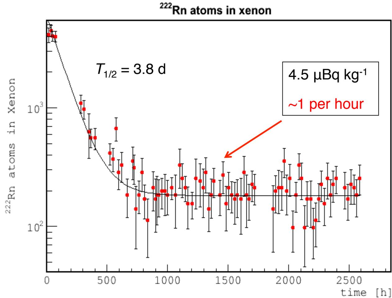
The <sup>214</sup>Bi decay rate is consistent with measurements from alpha-spectroscopy and the expected Rn background with no Rn trap.
