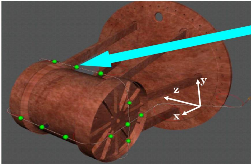
Calibration sources are deployed through a guide tube that wraps around the copper vessel
