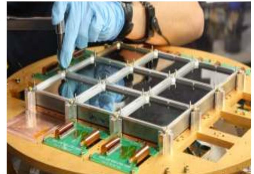
Plug & play detector modules each have 64 dual-pol 95 GHz camera pixels and contain cold multiplexing electronics. Contain all of Keck in one receiver!
