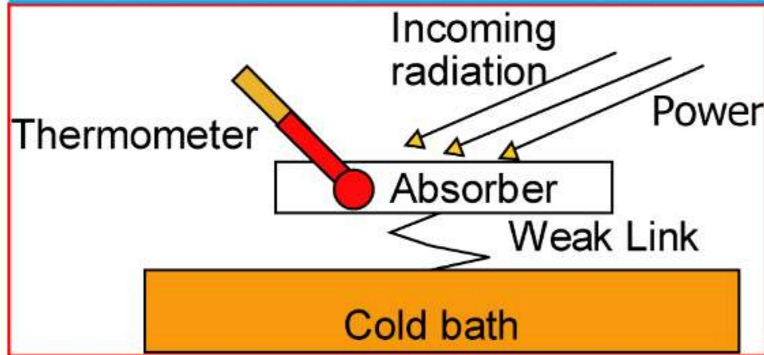
Sensors cooled to 0.25 K to reduce thermal noise
