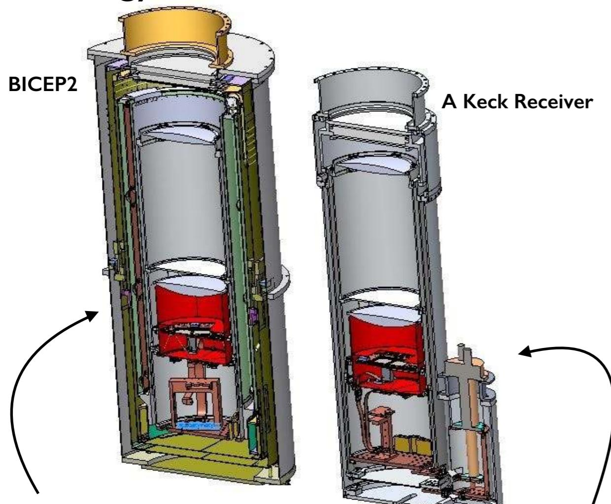
Keck receiver vacuum shell simplified compared to B2 for cryogen-free operation
